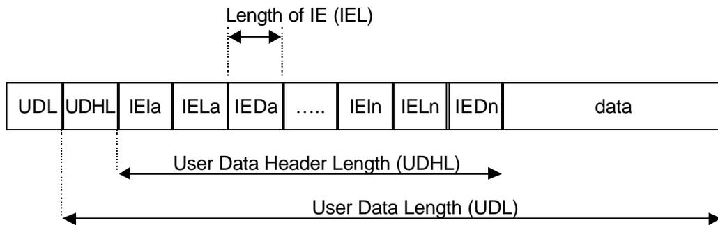
The UDH is always present when USSD is used as a transport mechanism for WAP.
