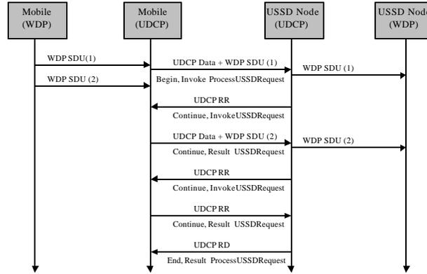
Figure 4 Example of WDP and UDCP inter working.
