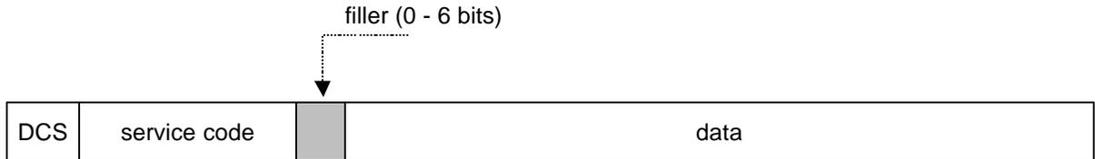
The service code, which is the only data the network is interested in, is encoded using the SMS default alphabet (7-bit characters), and it MUST comply to the GSM 02.90. The data starts on an octet boundary; filler bits are inserted between the service code and the data if needed.
